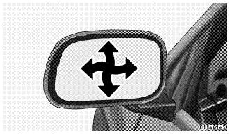
To adjust a mirror, turn the control wand toward the left or right mirror positions indicated. Tilt the control wand in the direction you want the mirror to move. When you are finished adjusting the mirror, turn the control to the center position to prevent accidentally moving a mirror.
